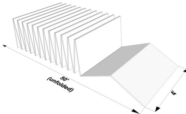
Figure 2. Duro-Guard XPS Fan Fold – K Dimensions
