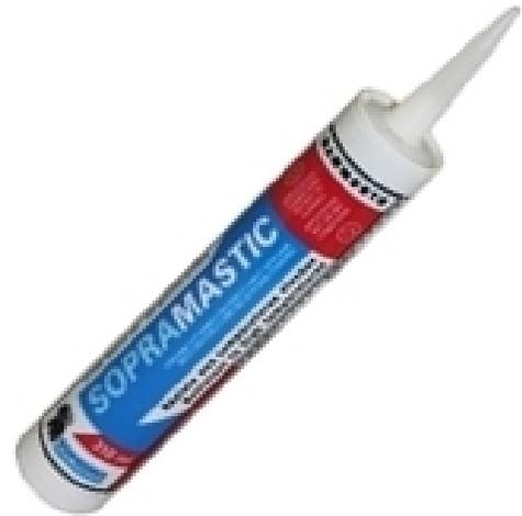
2. When Duro-Last Vapor Barrier is used as a temporary roof, apply Sopramastic at all T joints, transitions, and openings with a standard cartridge extruder gun. Sopramastic is not required if the Duro-Last Vapor Barrier is immediately covered by a complete roof assembly. **Sopramastic can be applied to damp surfaces.**
