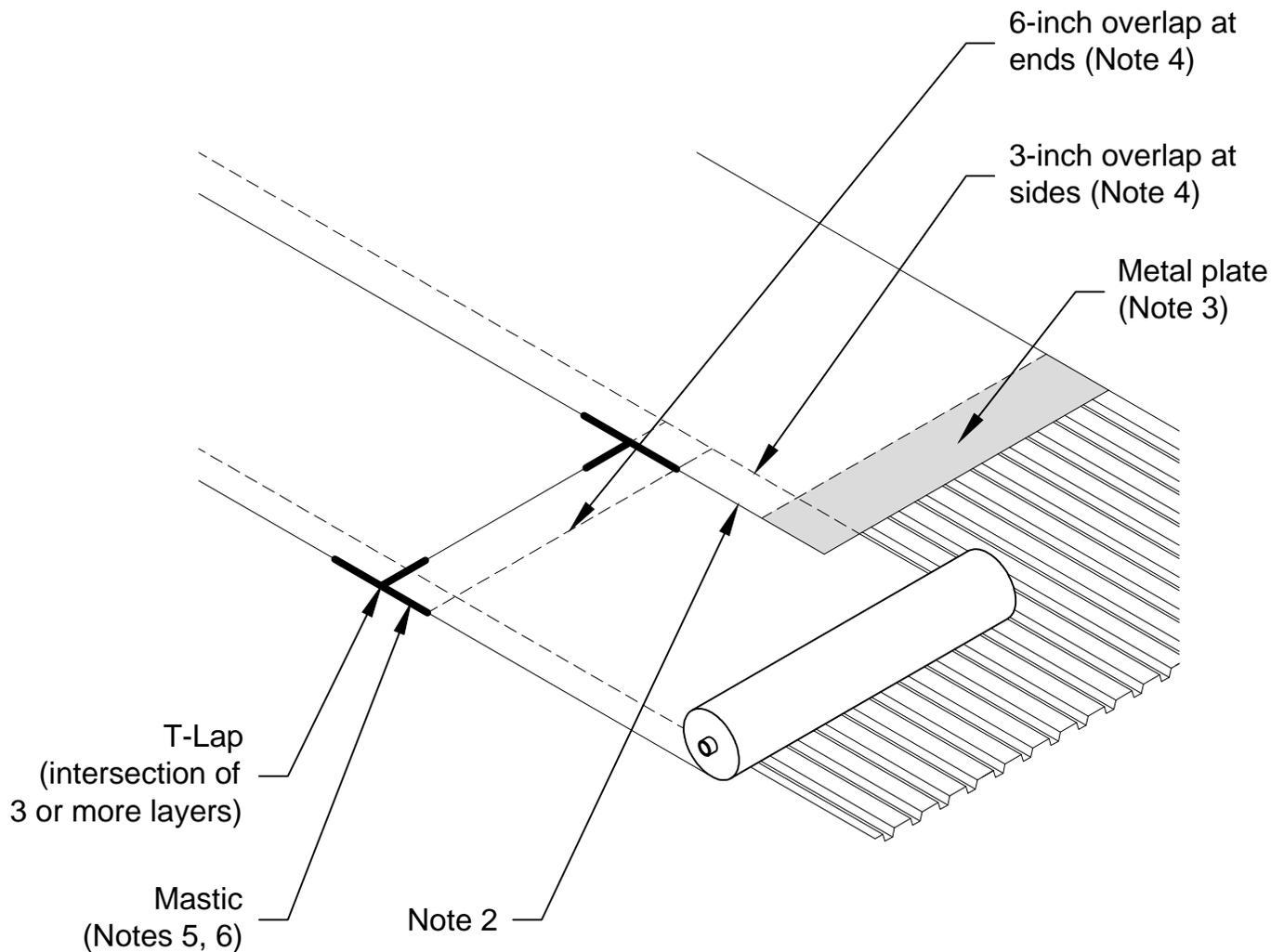
Note 1: Primer is not required when roof system is mechanically fastened or when substrate is a metal deck. All other substrates require primer.
