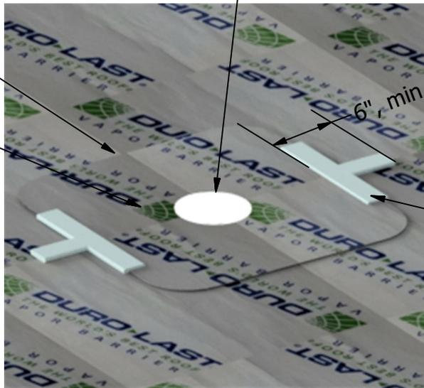
Cut hole 1/2 inch diameter smaller than penetration
