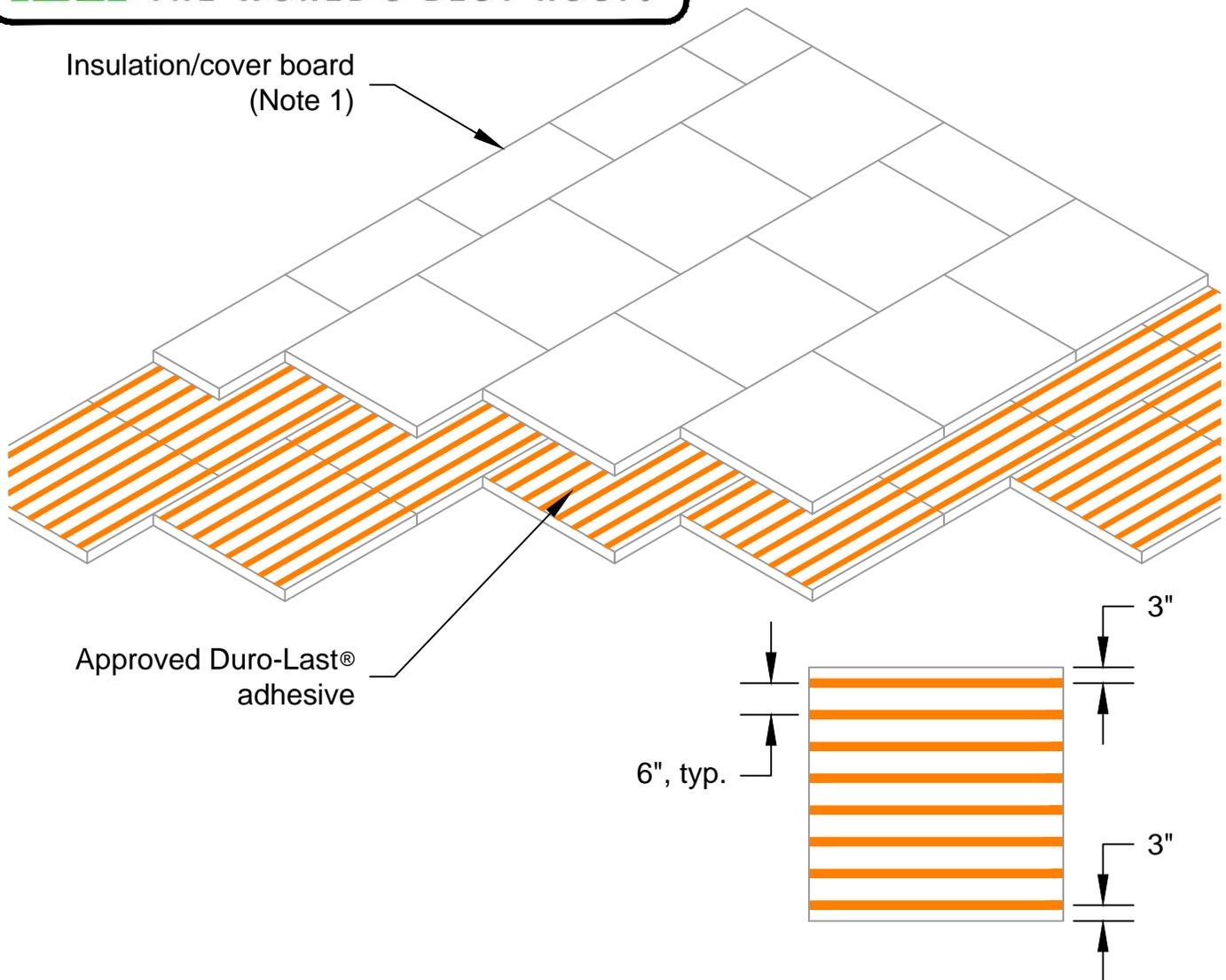
Note 1: Insulation must be no greater than 4 x 4-foot. Cover board must be no greater than 4 x 8-foot.
