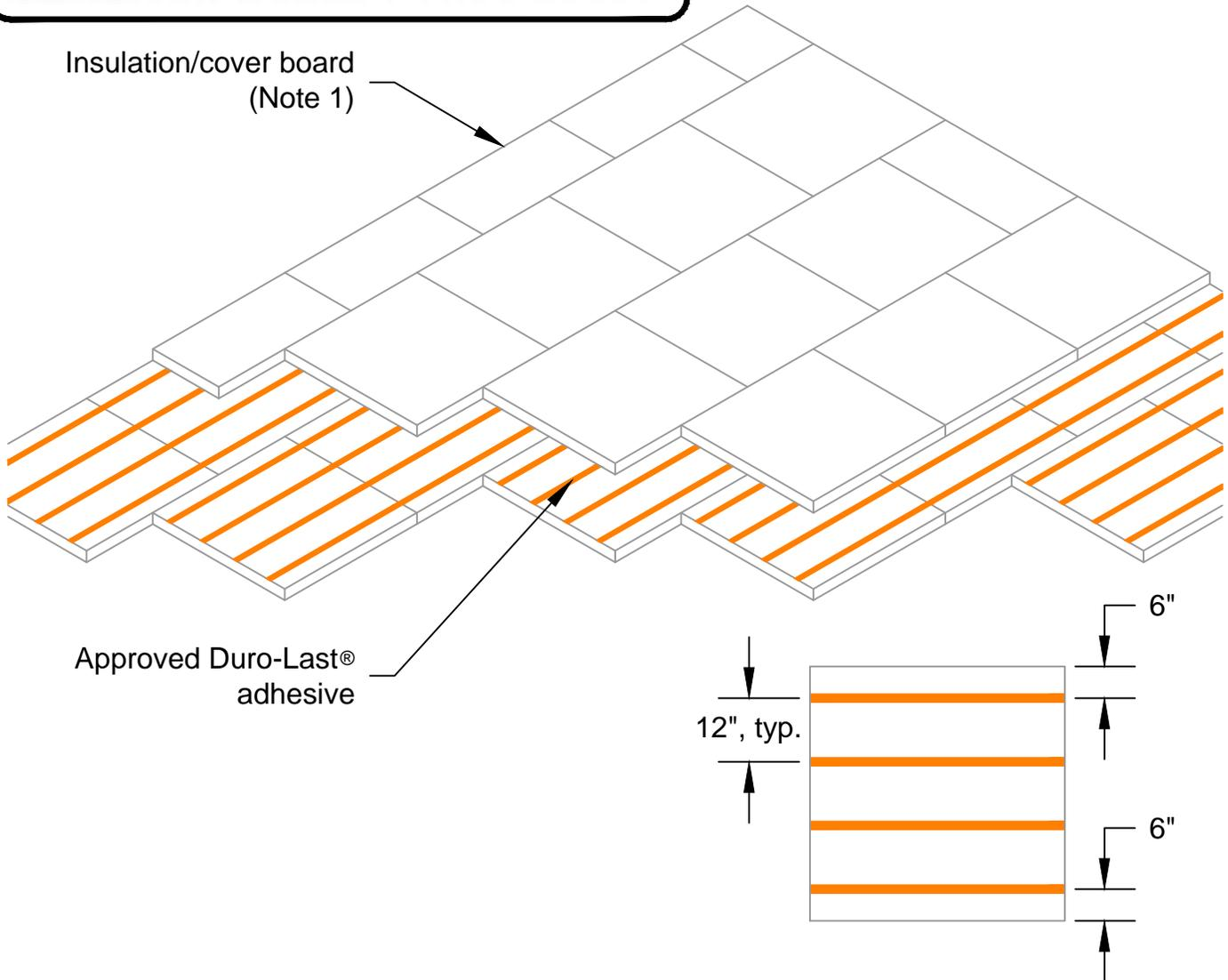
Note 1: Insulation must be no greater than 4 x 4-foot. Cover board must be no greater than 4 x 8-foot.
