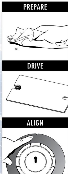
**1** Mark location where PowerGrip Plus is to be installed. Prepare membrane surface at each location following roof system manufacturers' requirements.
