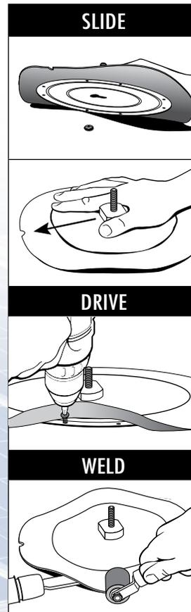
**4** Slide the PowerGrip Plus into place over the head of the fastener.
