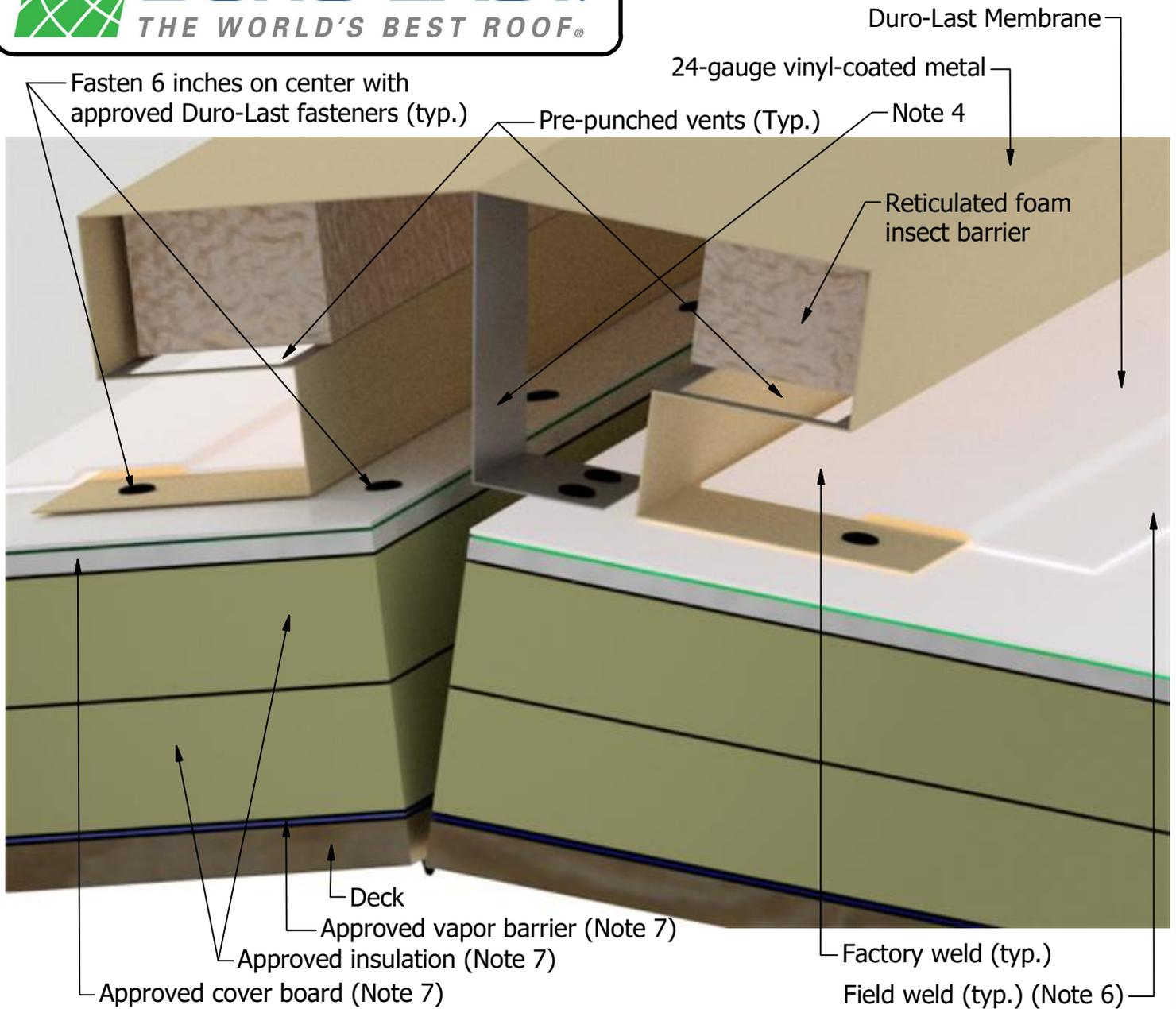
Note 1: Vented Ridge Cap comes in 10-foot lengths with a factory-welded 6-inch skirt on each side. Splice plates are used to join sections.
