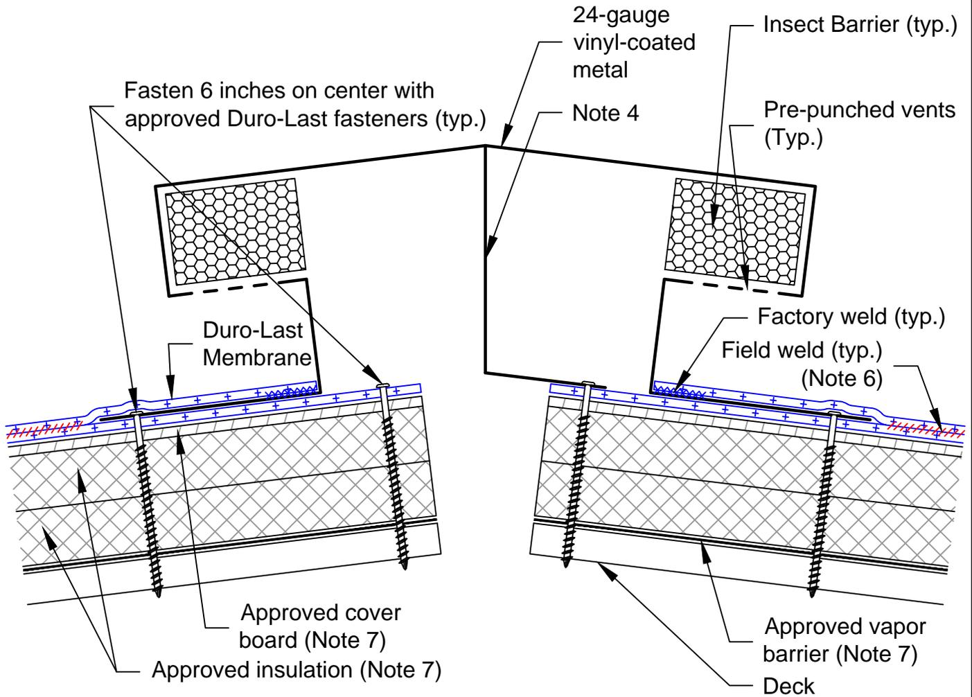
Note 1: Vented Ridge Cap comes in 10-foot lengths with a factory-welded 6-inch skirt on each side. Splice plates are used to join sections.
