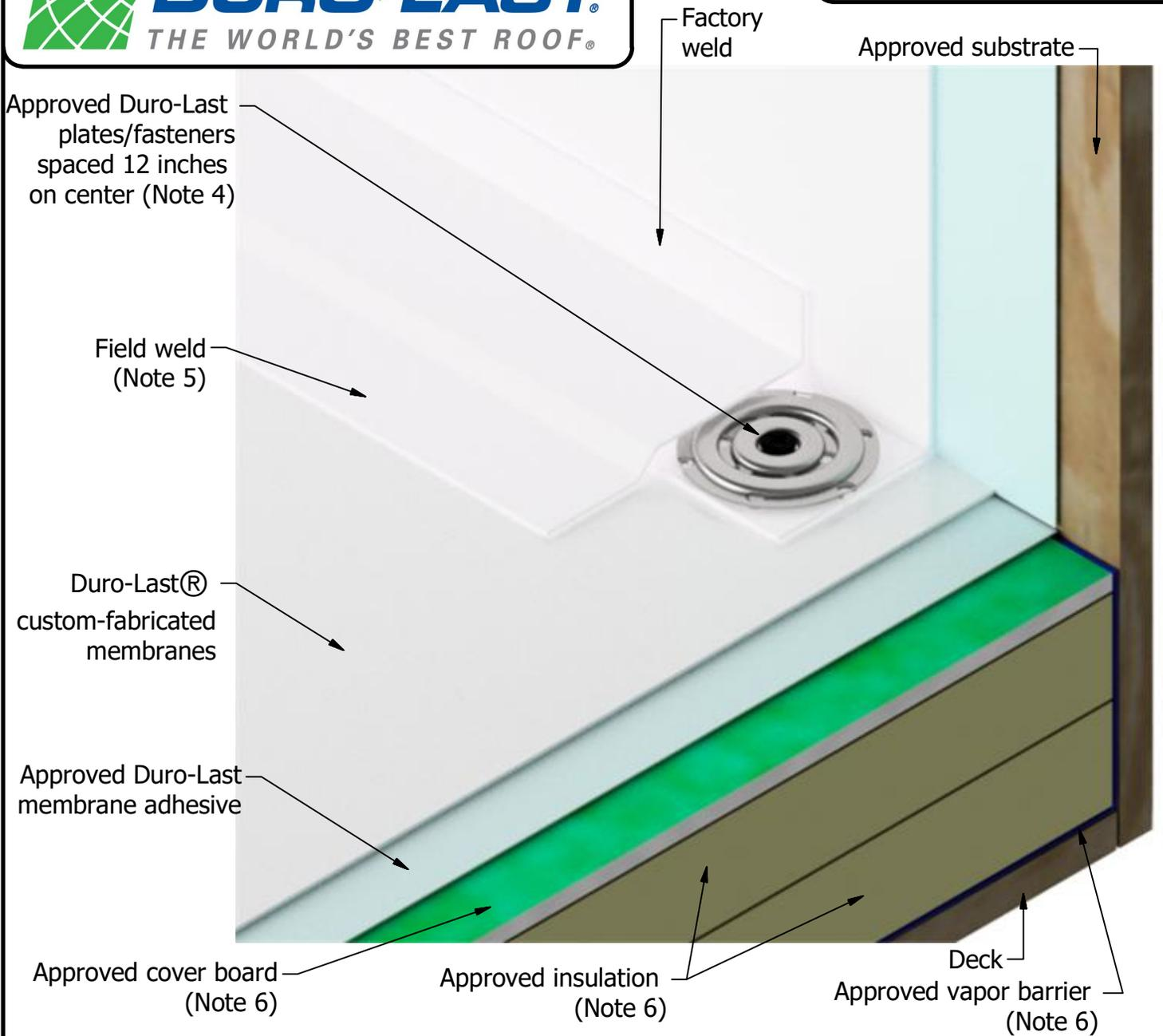
Note 1: When deck membrane is adhered and wall membrane is mechanically fastened, refer to Detail Drawings AS6000 and AS6001.
