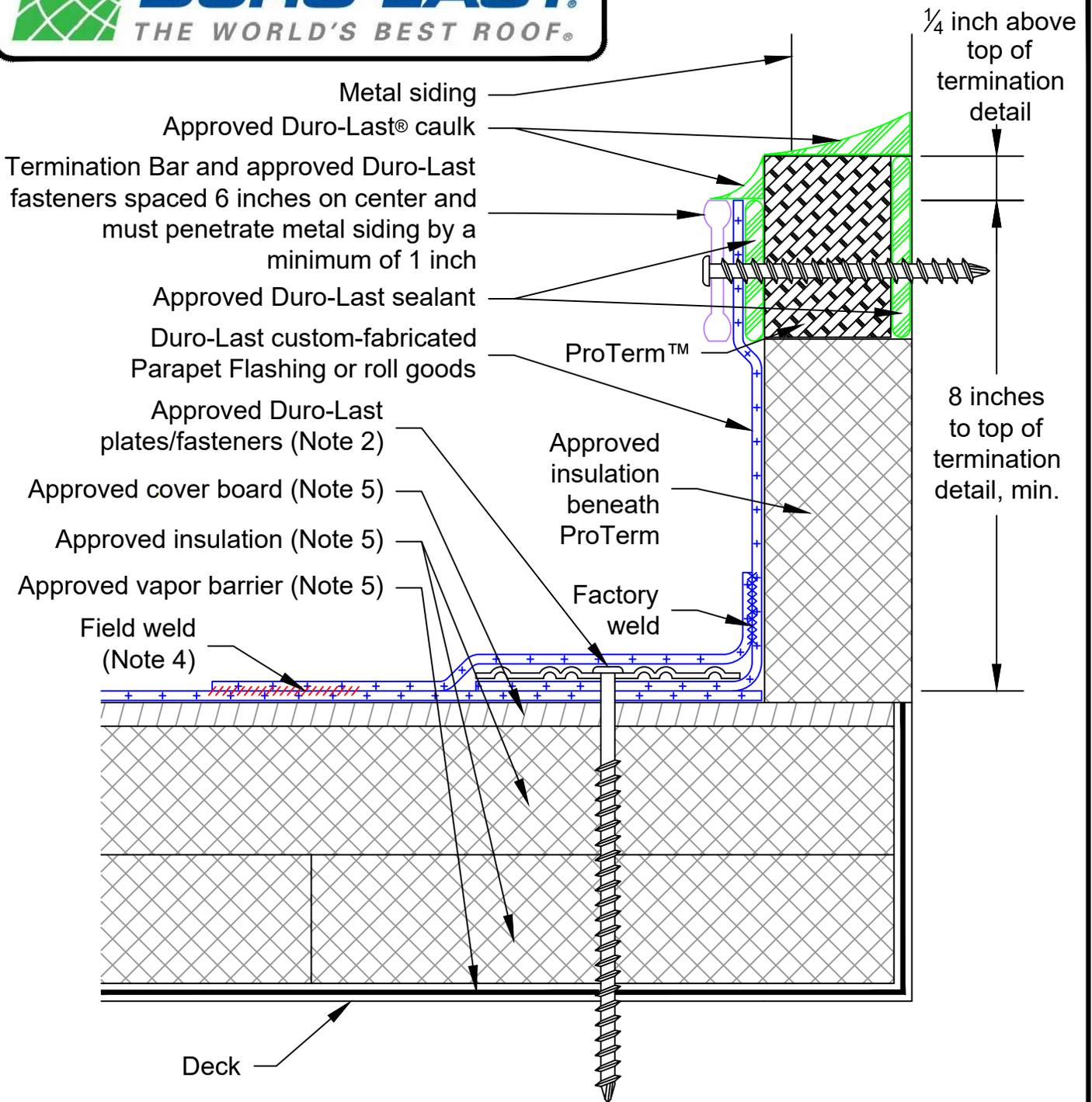
Note 1: Aluminum Termination Bar, 1-3/4 or 4-inch Fascia Bar and Cover (cover optional) may be used in place of Termination Bar.
