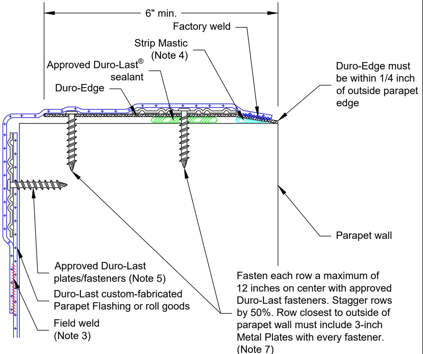
Note 1: This detail can only be used on parapet walls when termination over the parapet wall edge is not permissible or possible.
