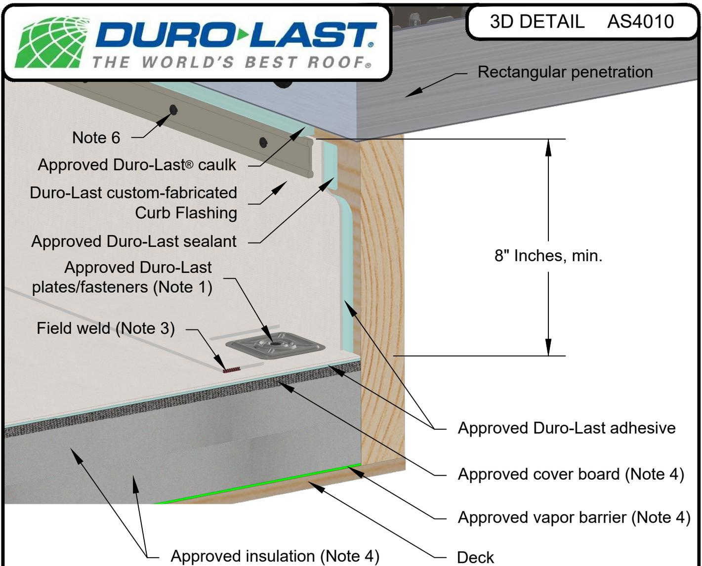
Note 1: Deck membrane shall be fastened around perimeter of roof penetration as per respective zone the roof access hatch is located within (field, perimeter, corner).
