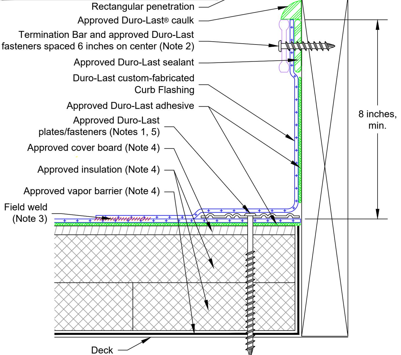
Note 1: Deck membrane shall be fastened around perimeter of roof penetration as per respective zone the rectangular penetration is located within (field, perimeter, corner). As an alternative to deck fastening, plates/fasteners may be fastened to the curb.
