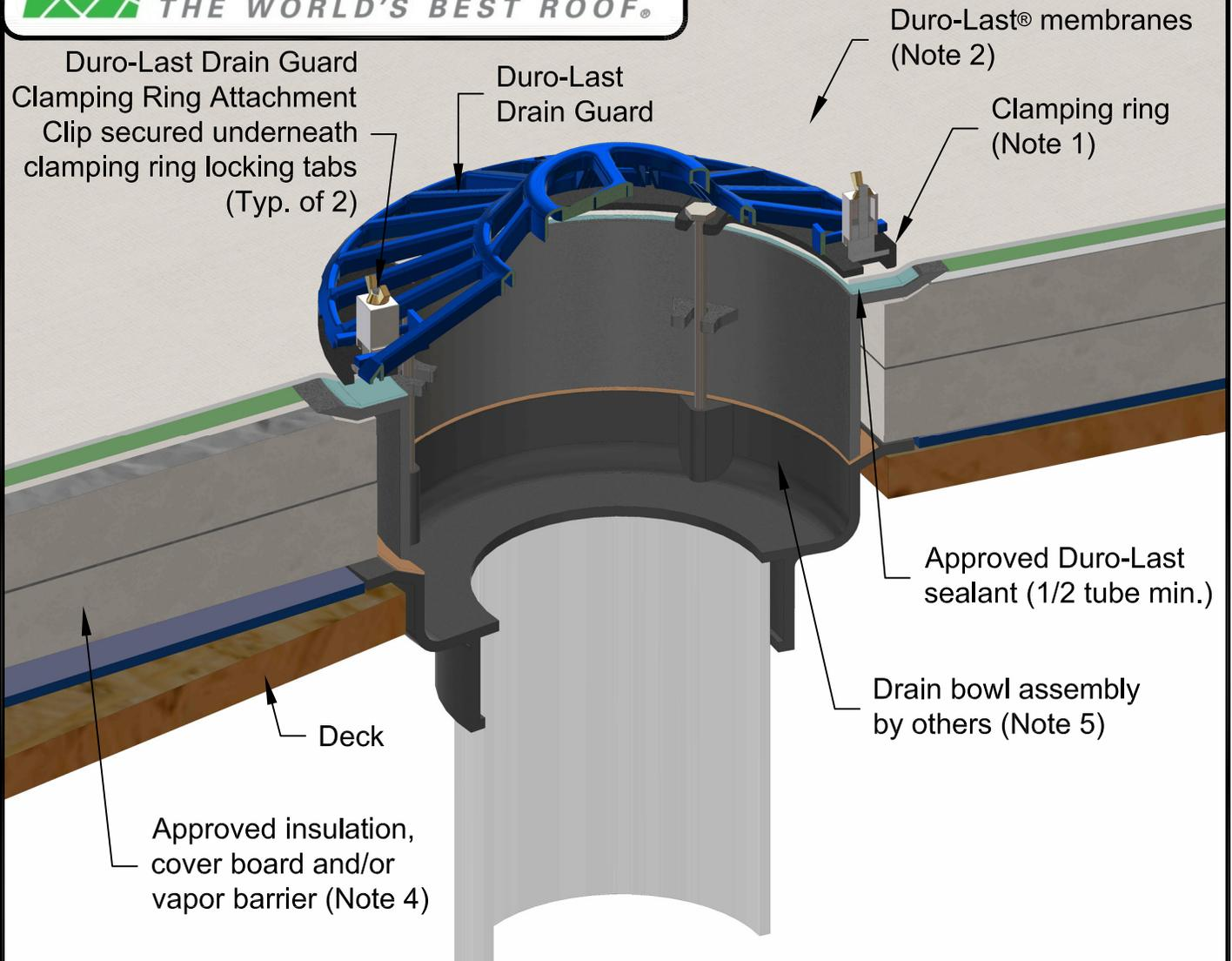
Note 1: Compatible clamping rings: Watts B2-FLG, Zurn 56588, Zurn 29480, Wade W-3000-I-FRG, JR Smith 3260 and JR Smith 35400.
