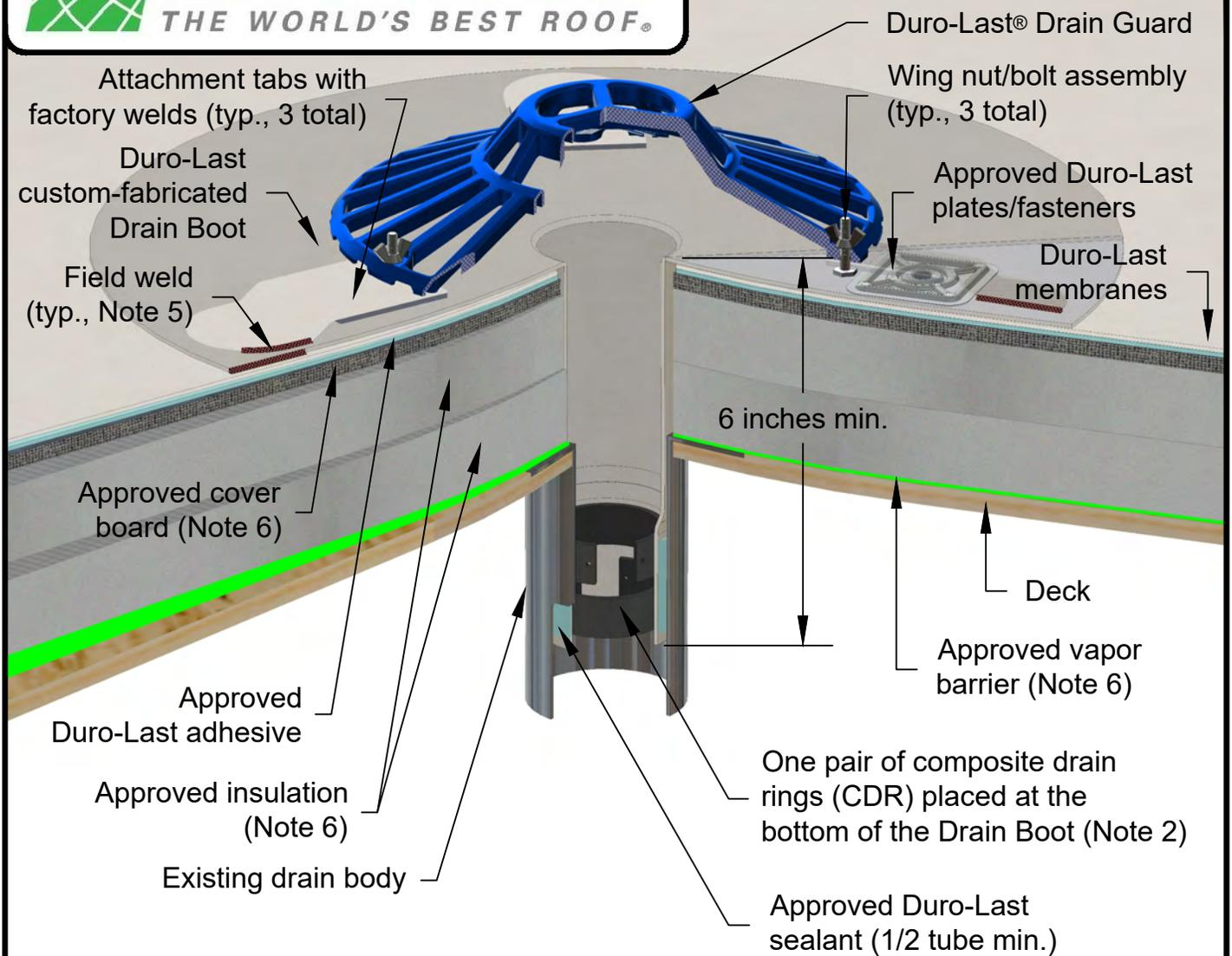
Note 1: Membrane must be fastened around the perimeter of the drain with the same fastening pattern as the field membrane, no less than 1 fastener per drain.
