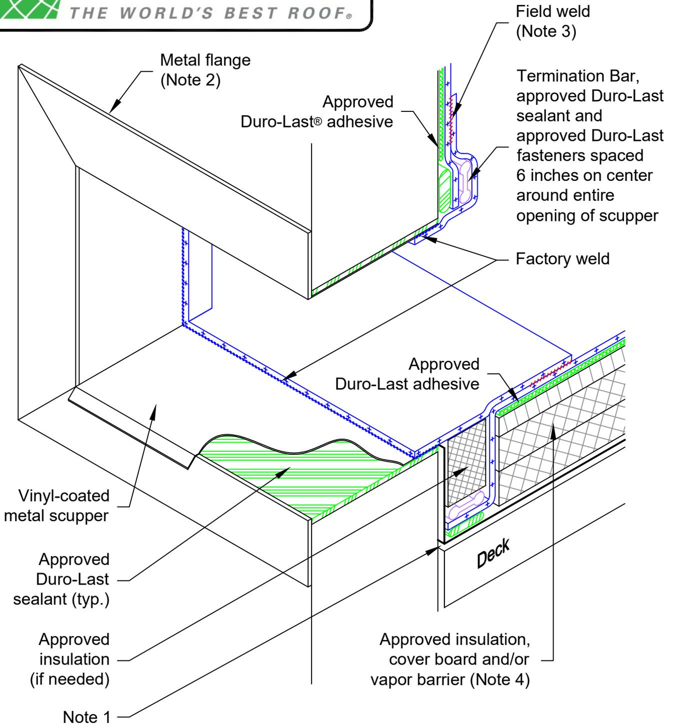
Note 1: Precaution must be taken to ensure that all wall-to-deck transitions are sealed.
