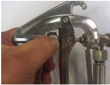
Spray gun control wheel adjustment
