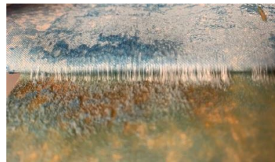
Acceptable adhesive “legging/stringing”
