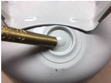
Location of rupture plug
