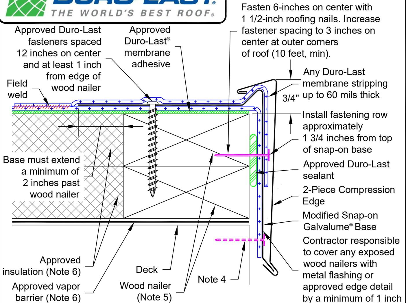
**Note 1: Detail Drawing AS9060C may be used in lieu of Detail Drawings AS9060A and AS9060B, but not within special wind regions or on parapet walls, when a peel stop is required. Refer to Detail Drawing AS9060 for peel stop requirements.**
