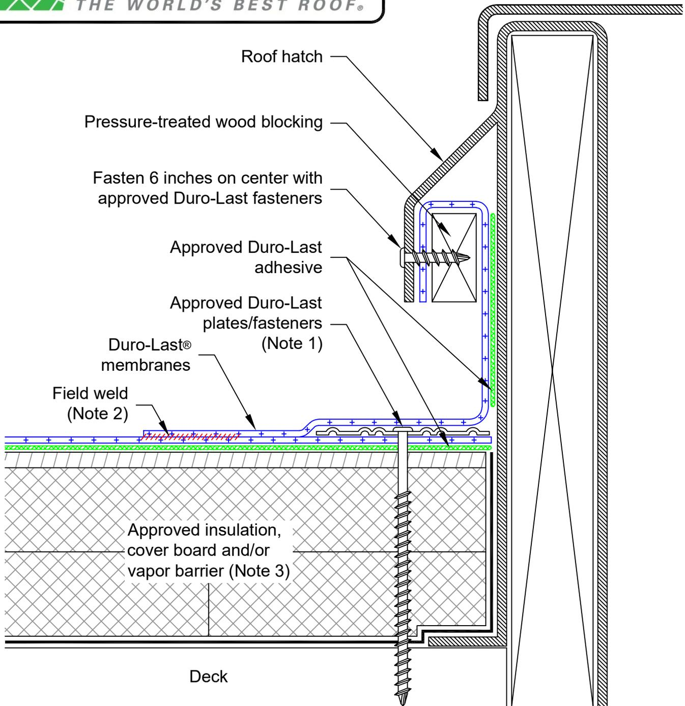
Note 1: Deck membrane shall be fastened around the perimeter of the roof access hatch as per the respective zone the roof access hatch is located within (field, perimeter, corner).
