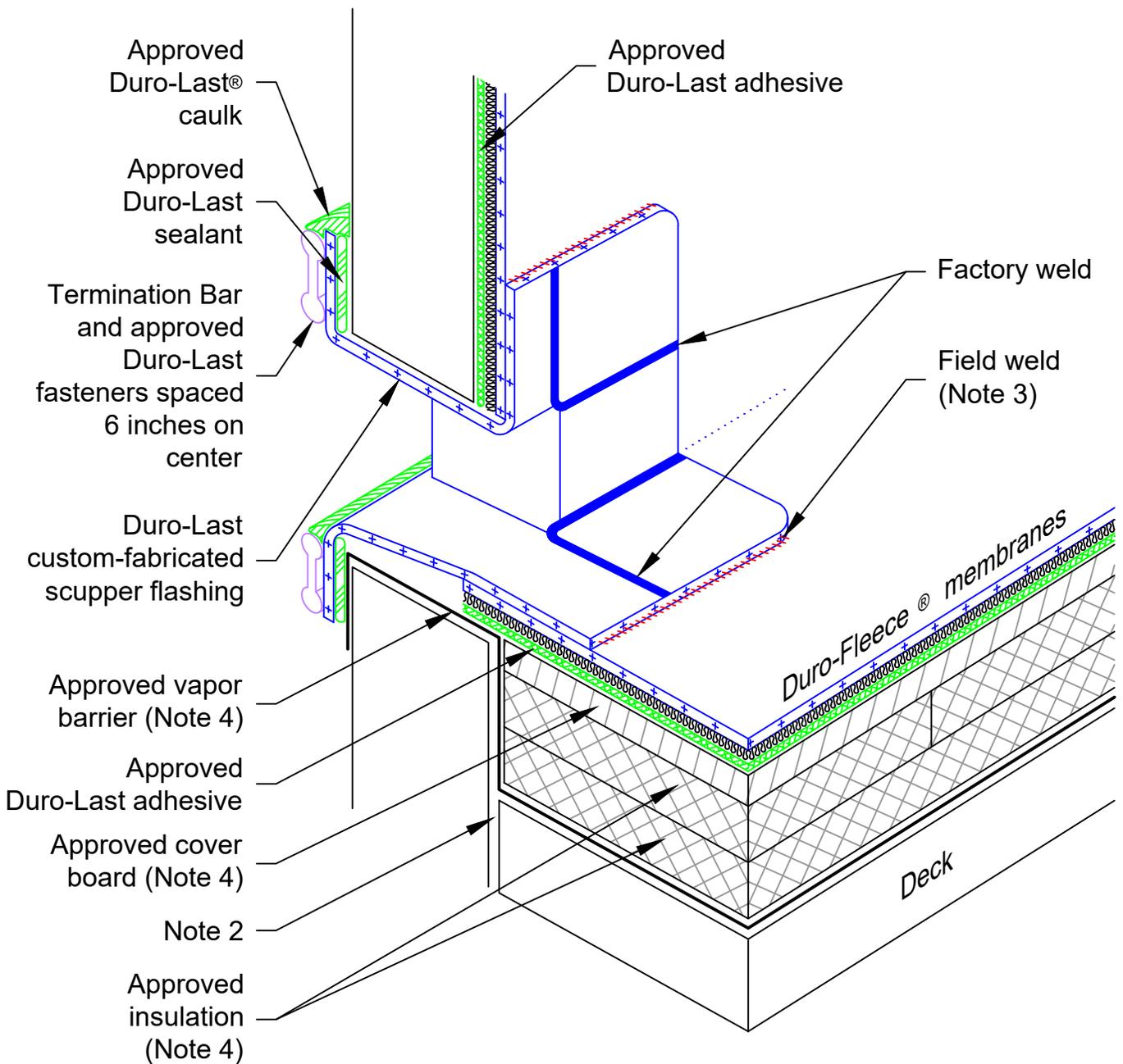
Note 1: Deck and wall membrane must be fastened around the perimeter of the scupper opening as per the respective zone the scupper is located within (field, perimeter, corner), no less that one fastener per side.
