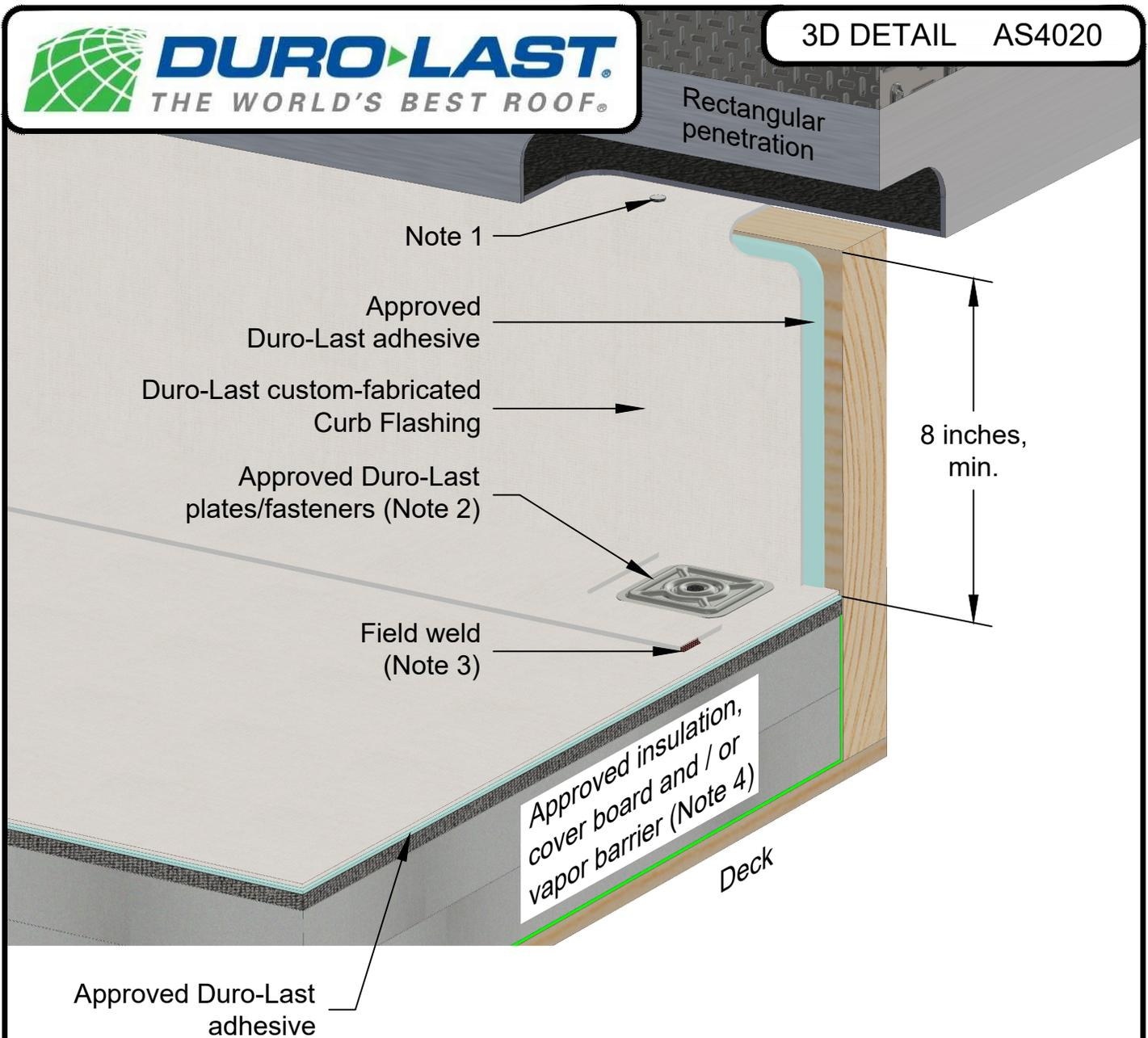
Note 1: 1 1/4-inch roofing nails spaced 6 inches on center.
