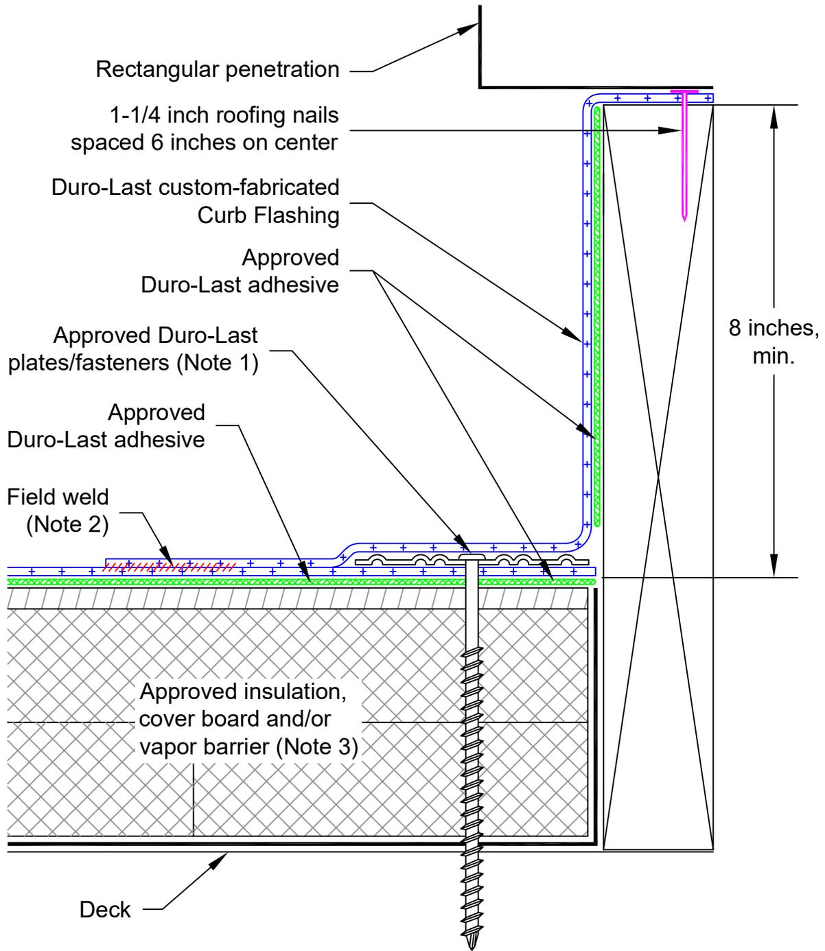
Note 1: Deck membrane shall be fastened around perimeter of roof penetration as per respective zone the penetration is located within (field, perimeter, corner).
