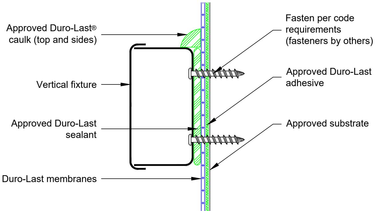
Note: Bottom of vertical fixture shall be a minimum of 8 inches above the finished roof deck.
