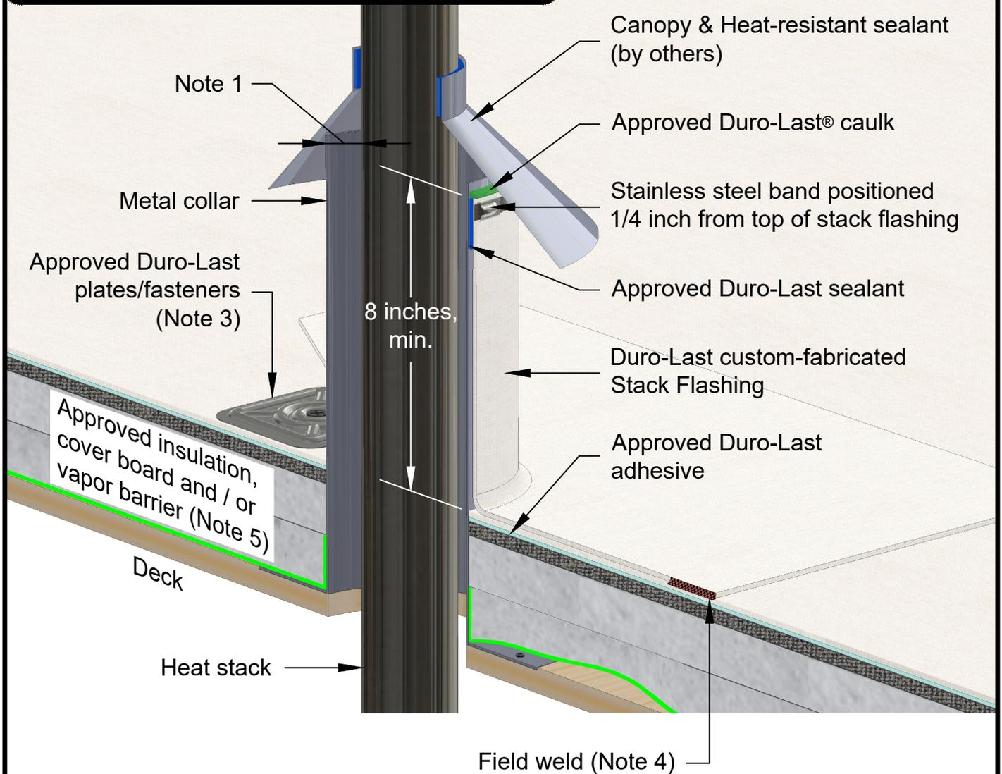
Note 1: This detail is required around heat stacks that exceed 120° F, including all insulated chimney stacks. A minimum of 1-inch air space is required between the metal collar and heat stack. The canopy must be positioned to allow adequate air flow above the termination.
