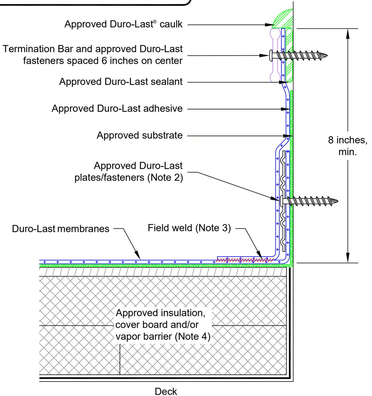
Note 1: 1-3/4 or 4-inch Fascia Bar and Cover (cover optional) may be used in place of Termination Bar.
