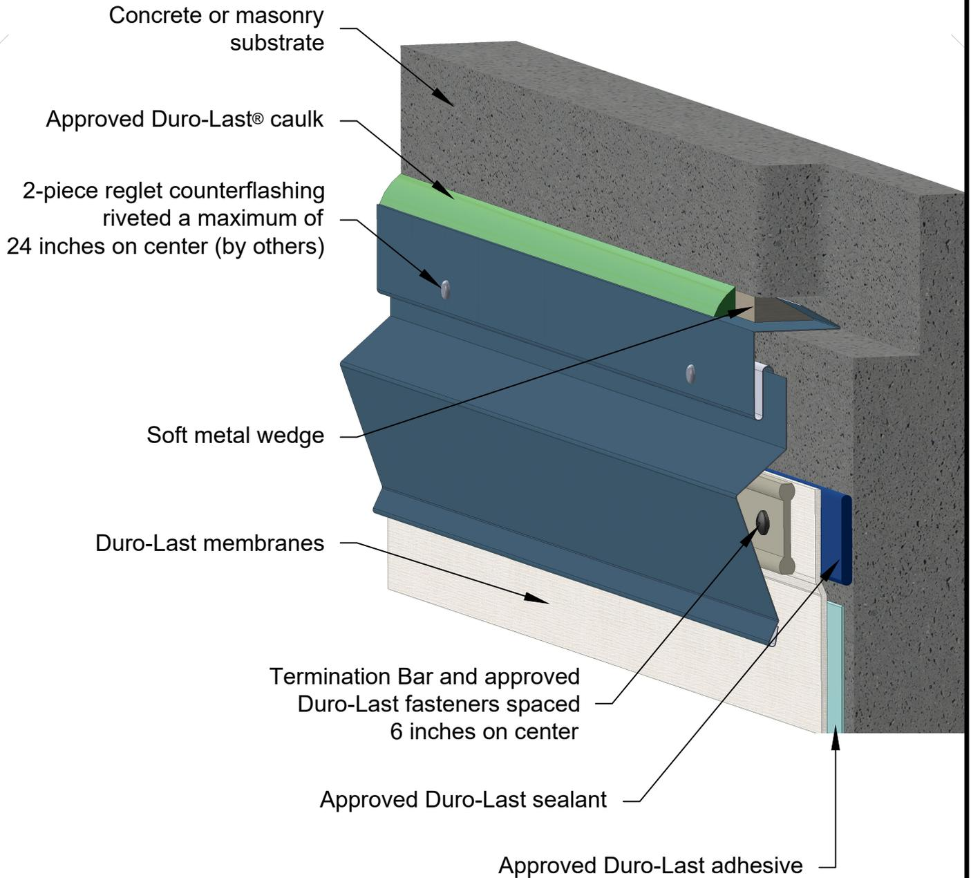
**Note 1: This detail is only applicable with concrete or masonry walls.**
