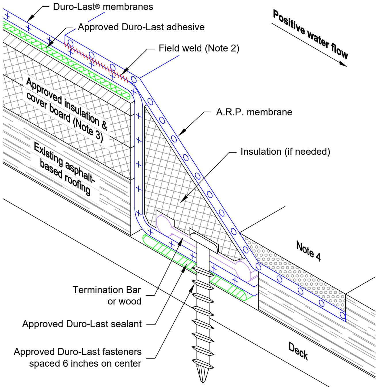
Note 1: Tie-in detail for all flat surfaces. The use of Detail Drawing AS1070 will be required in conjunction with Detail AS1080 when tie-in is across metal flutes.
