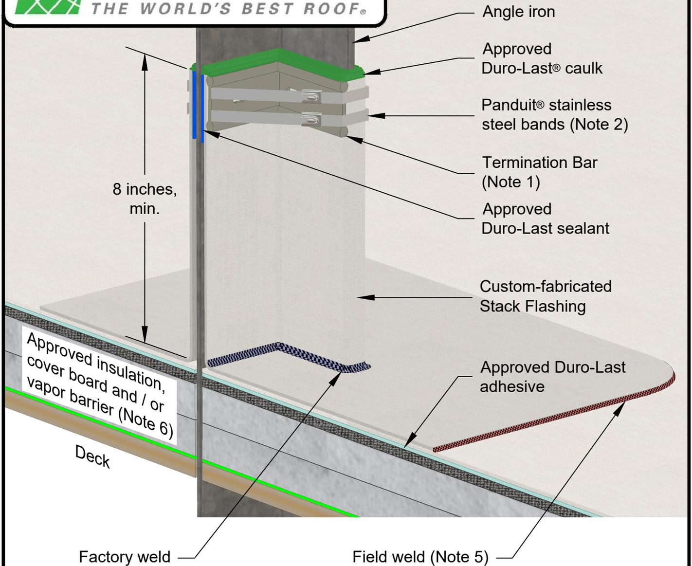
Note 1: Cut Termination Bar slightly larger than side of angle iron to allow for compression of Termination Bar by Panduit bands.
