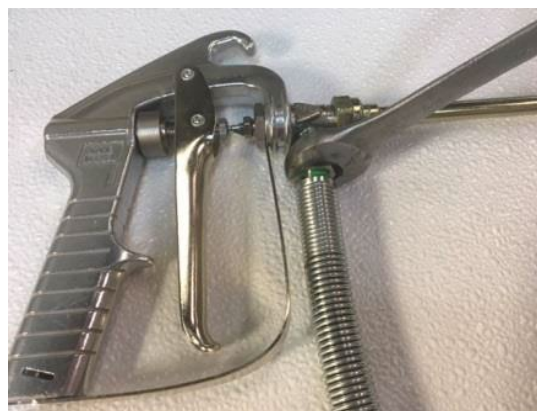
Hose to spray gun connection
