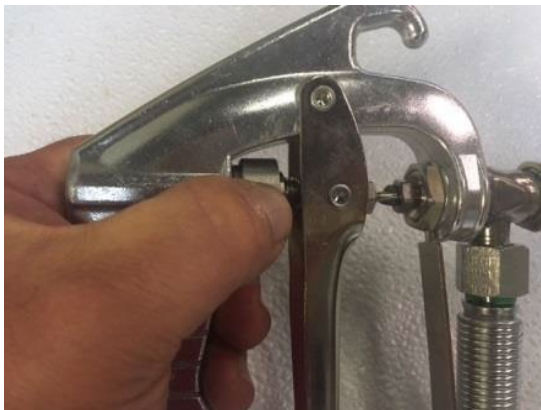
Spray gun control wheel adjustment
