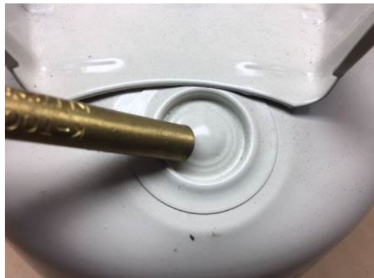
Location of rupture disk
